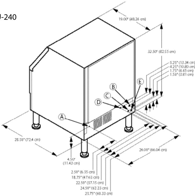
**Installation Note** Recommended clearance for top, sides, back is 5" (12.7 cm) however, there is no minimum clearance required.
